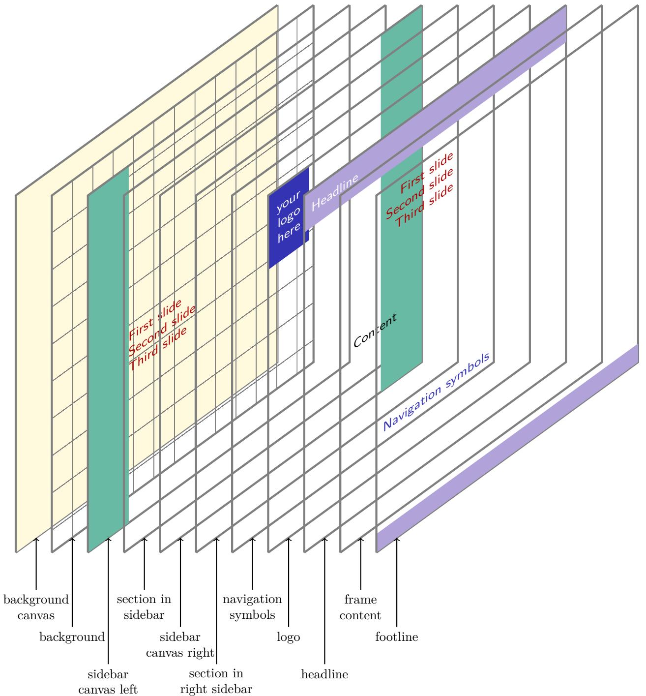
Figure 1: Diagram of the order in which the different frame components are drawn (image originally created by [Andrew Stacey](#))
